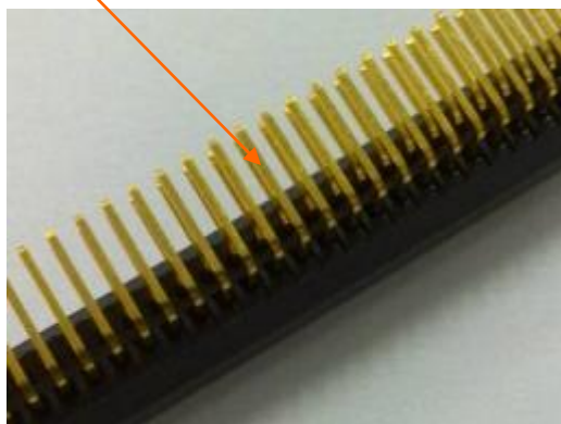
Yellow color at solder tail area
