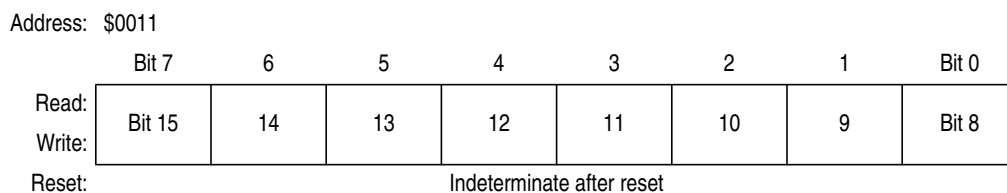
Figure 8-12. TIM Channel 0 Register High (TCH0H)
