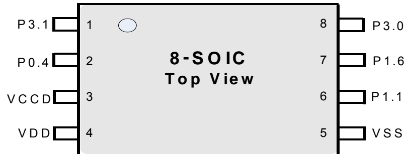
Figure 6. 8-Pin SOIC Pinout
