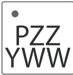
Figure 15 ■ Package Marking Specifications for PE42424
